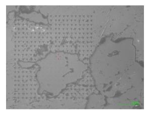
Indents to 20 mN of load in silicate rock with a height (hardness) contrast. Smaller indentation marks are due to the increased hardness on the "islands".
