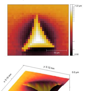
Plot of the topography obtained from surface detection height using Gwyddion. It can be visualized, using the nonlinear color scale, that the deformation extends much further than visible in the optical image.
