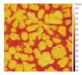
Mapping the elastic modulus shows two separate phases corresponding to optics. Histogram plotted below.
