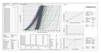
Results indicated in software with 10000 load-displacement curves showing full set of data.
