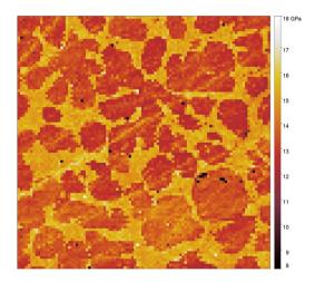
Reversed contrast for hardness of the phases. Hardness varies also due to scratches, contaminations, imperfections.
