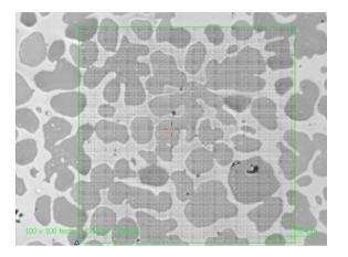
Co-Al intermetallic phases visible in optical microscopy image of the polished surface. Green overlay: 200x200 µm with 100x100 indents.
