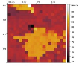
Mapping the elastic modulus shows a distribution, which correlates with the optical observations.
