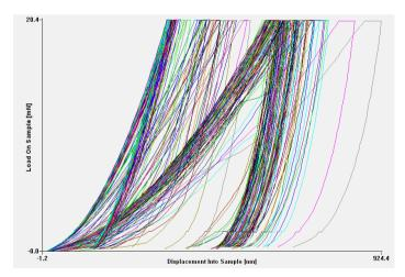
Low cycle time testing allows to study and to compare the indentation curves for all indents. The two groups of curves show the two hardness levels within the mapped sample region.
