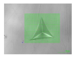
In order to study the topography of the Berkovich imprint, an array of 30x25 indents with a spacing of 5 µm was placed on the imprint. We used a cubecorner tip for best imaging and limited the indentation load after surface detection to 50 µN.
